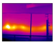
colors. The fire "seam" is located along a weld joint around the circumference of the silo and is approximately 5' in depth. This fire is approximately 12' down from the surface of the coal.
