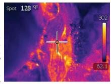
Actual images from the power plant bunker fire with a thermal imaging camera identifying the coal hot spot.
