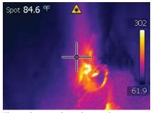
Thermal image shows heat reduction during F-500 EA piercing rod treatment.
