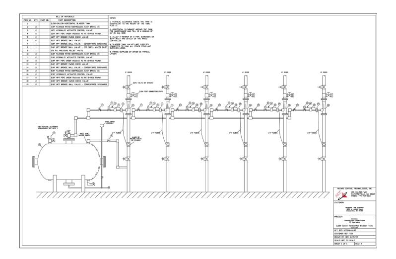
The F-500 Encapsulator Agent Concentrate Control Supply systems with 3% ratio controllers, were commissioned, tested and approved. The system is based on a 2600 gpm water flow and 30 minutes of enhanced and properly proportioned F-500 EA to protect the under turbine lube oil and transformer areas from fire.
