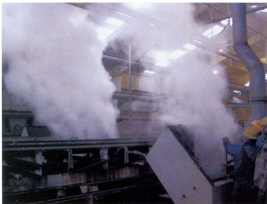
2. Smoke means fire. Immediate response is required when an odor of coal roasting or burning is detected as coming from a silo, bunker, or hopper. Delays in taking action only allow the rate of burning to increase. Courtesy: Utility FPE Group Inc.
