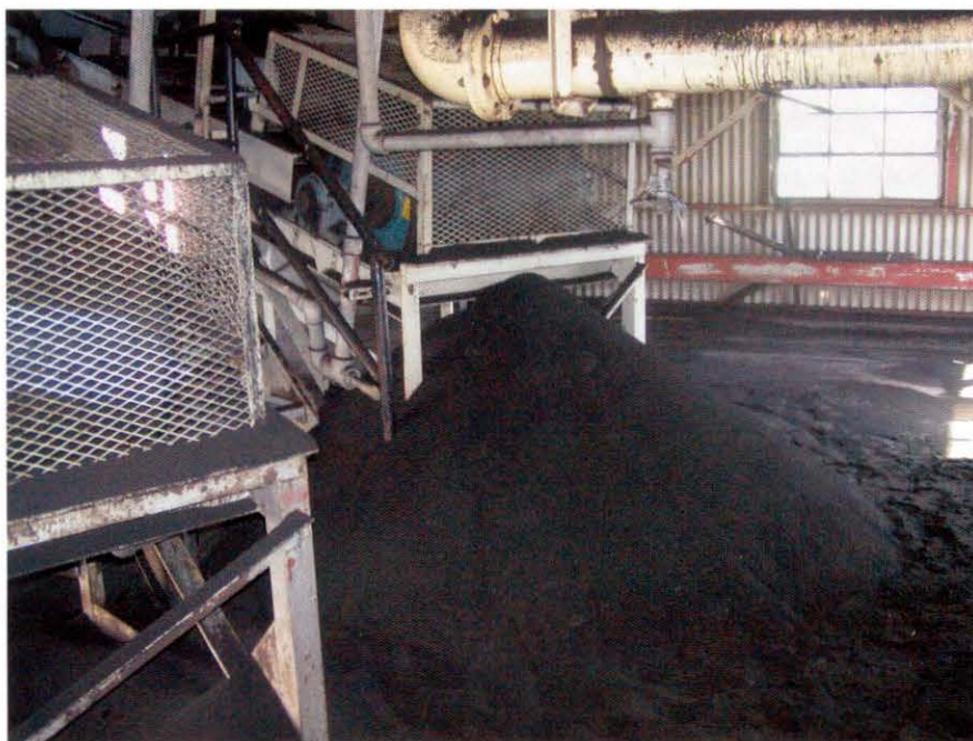
1. Debris dump. An extreme case of PRB coal accumulation at the tail of a conveyor not designed for PRB coal. Courtesy: Utility FPE Group Inc.
