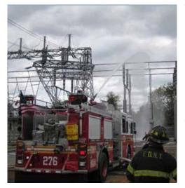
This incident led Con Edison to evaluate various firefighting agents for transformer fires. Only one agent was capable of being applied to 345 kV with imperceptible electrical feedback to the nozzle, F-500 Encapsulator Agent. Today, Con Edison recommends F-500 Encapsulator for transformer fires. After the power is removed, F-500 EA can be safely applied without fear of electrical feedback to the nozzle if the stream comes into contact with nearby energized peripheral equipment.
